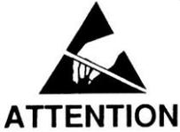
The Control Unit is susceptible to static voltage. Connection of a clean ground to terminal 31 is essential for optimum performance. Prior to this connection, static handling precautions should be taken.
