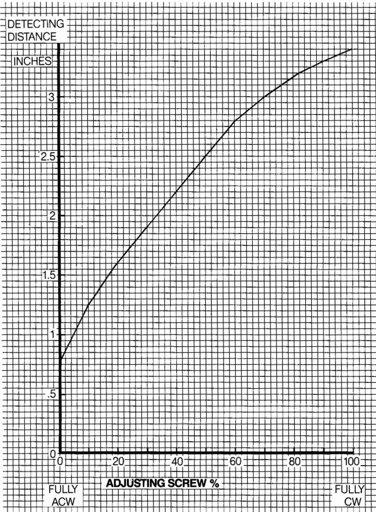
**MARK 2: MOTION PROBE SENSITIVITY WITH ADJUSTING SCREW**
