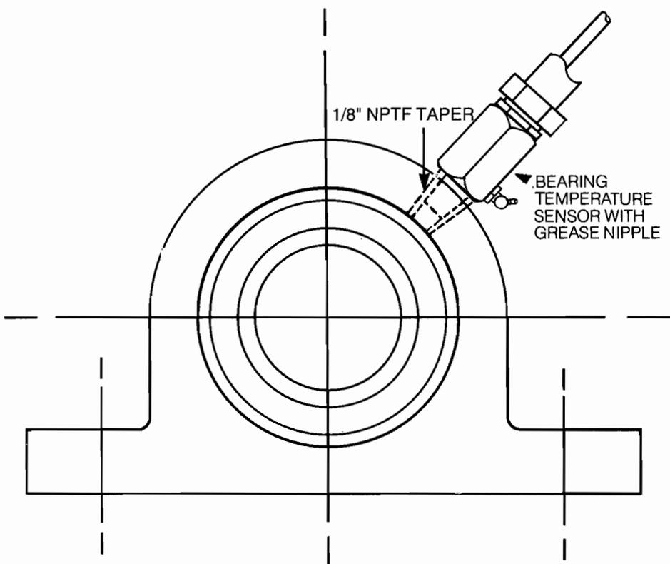
**FITMENT TO BEARING OF TEMPERATURE SENSOR**
