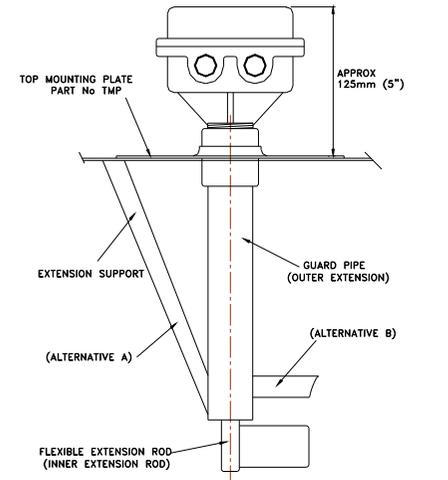
EXTENSION RODS AND GUARD PIPES CAN BE PROVIDED FOR LOW LEVEL OR WHEN RL'S ARE MOUNTED HIGH IN THE BIN/SILO ROOF
