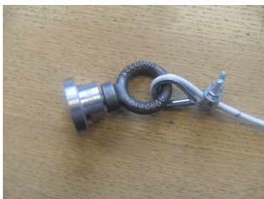
Steel rip wire with metal clamp
