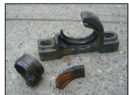
Example of Bearing Failure
