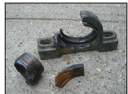
Example of Bearing Failure
