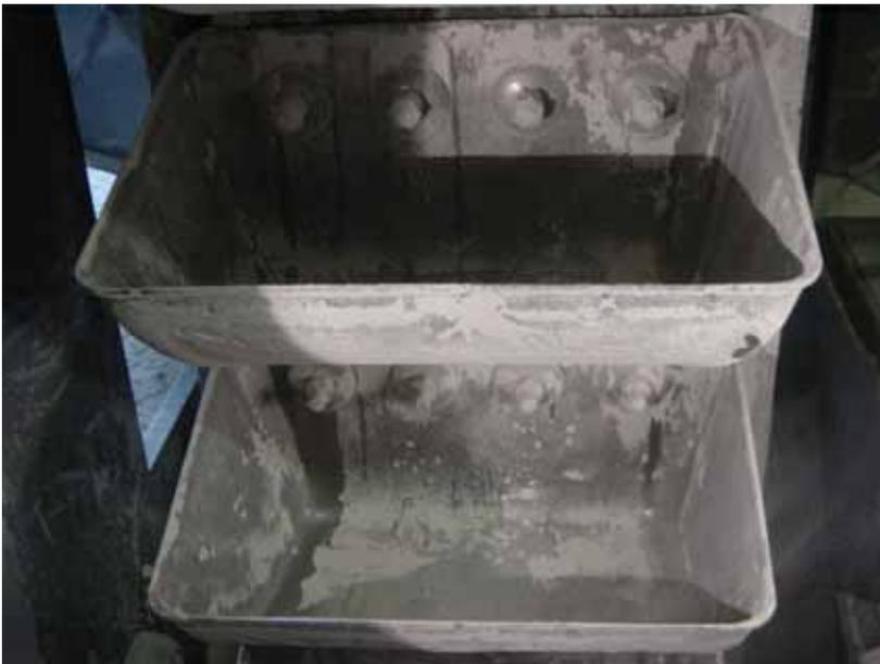
The next example is of an existing chain elevator in Australia that was upgraded from 120 TPH of cement, upto 250 TPH by retrofitting and installing one row of SJ470 buckets and using Ferro belt SW1000 4+4. The original elevator 25 meters high, had chain installed, and it was decided to change over to Ferro belt with SJ buckets to improve the performance and life.
