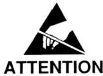
**The Control Unit is susceptible to static voltage. Connection of a clean ground to terminal 29 is essential for optimum performance. Prior to this connection, static handling precautions should be taken.**
