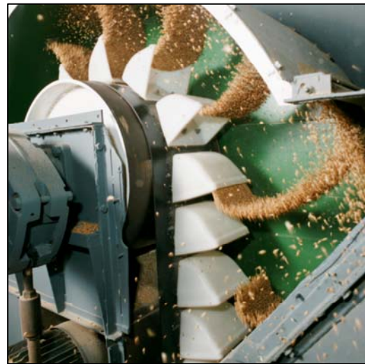
Centrifugal Discharge of CC-S Buckets Shown Handling Grain
