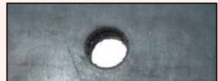
Clean cut hole
