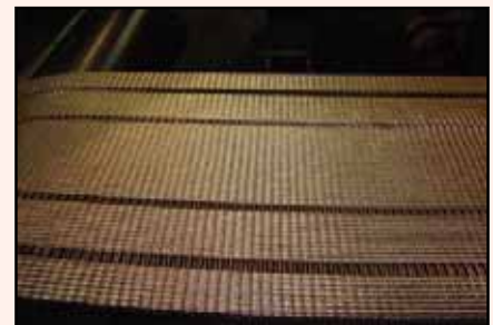
Carcass of Polysur® Ferro belt with cable free zones during production
