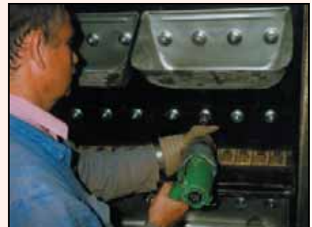
fitting buckets to the belt
