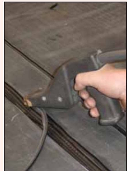
Rubbercut assembly for removal of cover rubber
