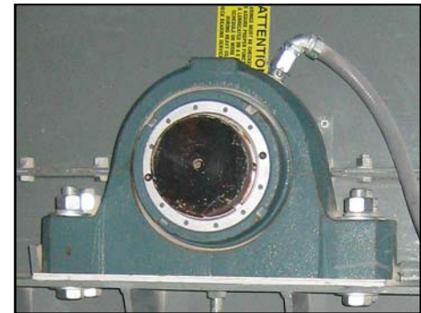
Bearing Sensor on Belt Conveyor
