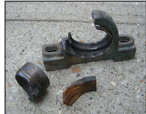
Example of Bearing Failure
