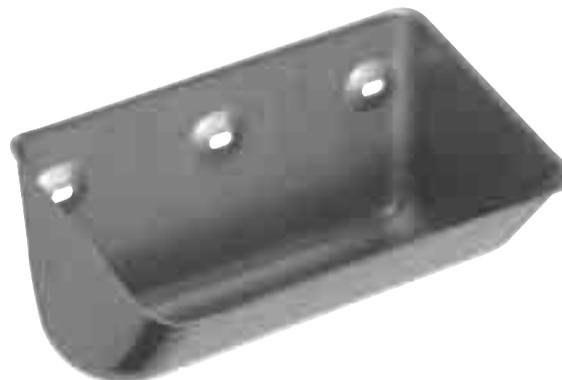
problem due to frequent operational exposure. Consideration should also be given to the style of fasteners used to mount steel buckets, which will also help protect the investment. Fanged or Norway bolts would be recommended with the use of a flat washer and nylon insert locknut, or the selected style elevator bolt with a large flanged wizz locknut. Both scenarios will provide the most secure holding power.
