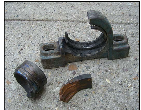
Example of Bearing Failure
