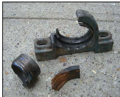
Example of Bearing Failure
