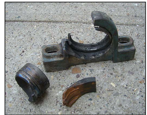
Example of Bearing Failure
