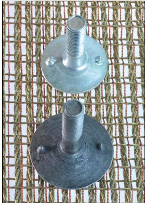
Bolt M12 with 50 mm head diam covers 25% more warp and weft cables than standard 42 mm head diameter resulting in stronger bucket to belt attachment.
