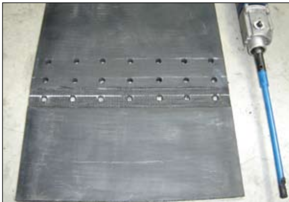
Clamp holes drilled and drilling tool.
