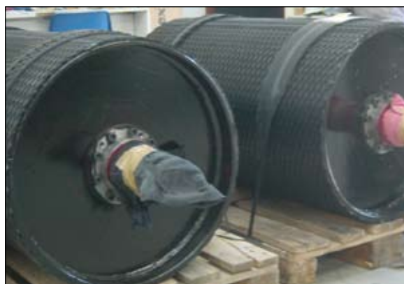
Replace drive pulleys.
