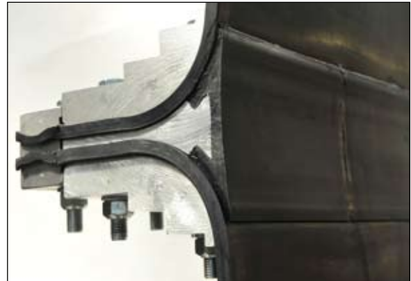
MB Solid belt clamp pulley side.
