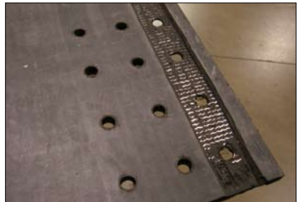
Belt end ready to fit clamp.
