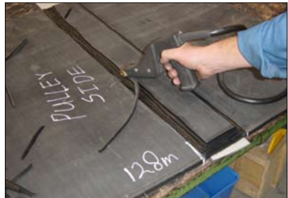
Preparing groove in belt end to fit vice-grip.
