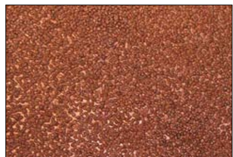
Sintered metal segments preformed to pulley face.
