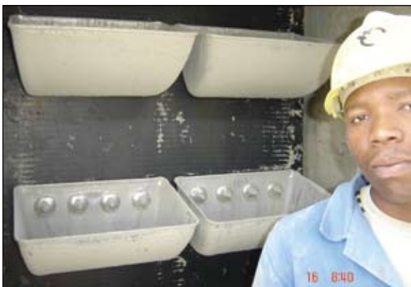
Light weight buckets in 2 rows handling 250 T/h cement on 850 mm wide belt.
