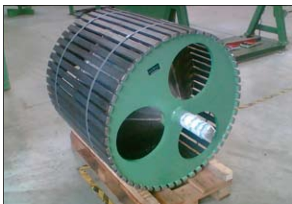
Replace slatted boot pulley.
